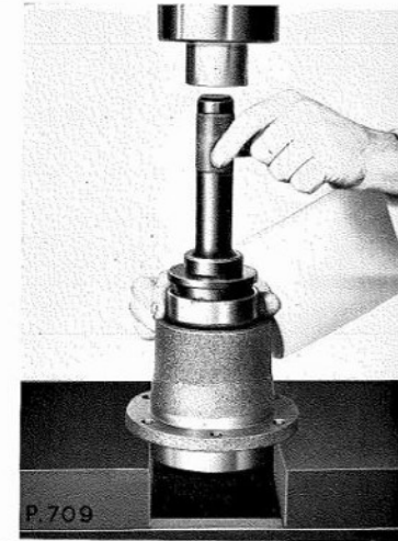
Fig. G.10. Pressing in the bevel pinion outer bearing cup, using the Churchill Tool R.G.323, in conjunction with the universal handle 550, applied in the normal position
