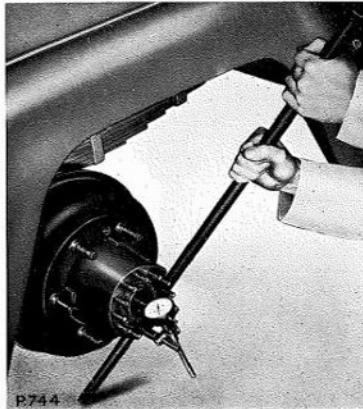
Fig. G.18. Checking the rear hub bearing for end float, using the Churchill Tool R.G.335, in conjunction with a dial gauge (1st checking operation illustrated)
