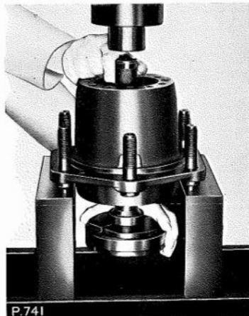
Fig. G.20. Pressing out the wheel hub inner bearing cup, using the Churchill Tool R.G.314, in conjunction with the universal handle 550
