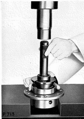
Fig. G.26. Pressing in the bevel pinion outer bearing cup, using the Churchill Tool R.G.315 in conjunction with the universal handle 550
