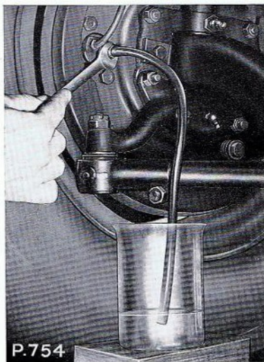
Fig. K.14. Bleeding the hydraulic system
