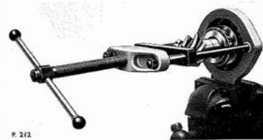
Fig. G.27. Fitting the bevel pinion inner bearing cone, using the Churchill Tool R.G.4221B and the adaptor set R.G.4221B-13
