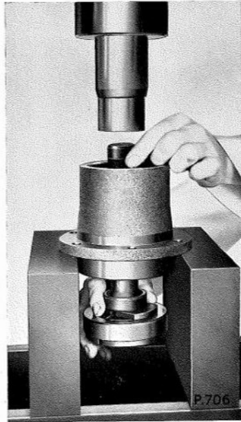
Fig. G.6. Pressing out the bevel pinion inner bearing cup from the bearing sleeve, using the Churchill Tool R.G.315, in conjunction with the universal handle 550, applied in the normal position
