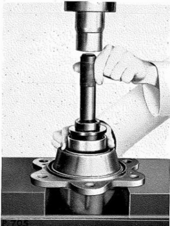
Fig. F.6. Pressing in the KA.30 front hub inner bearing cup using the Replacer Pad of Churchill Tool R.G.324 together with the Universal Handle 550
