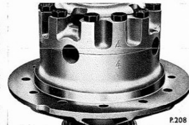
Fig. G.29. Identification marking on the differential case halves
