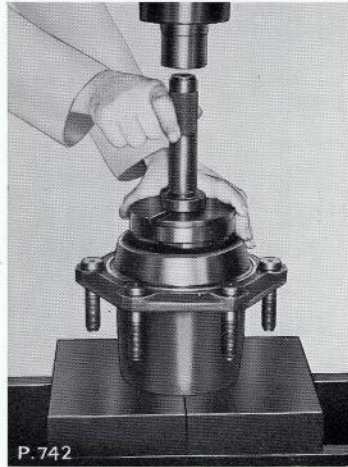
Fig. G.23. Pressing in the wheel hub inner bearing cup, using the Churchill Tool R.G.314, in conjunction with the universal handle 550
