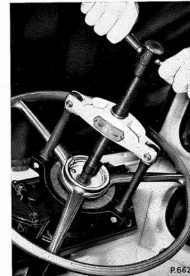
Fig. J.8. Removing the steering wheel using Churchill Tool R.G.3600 and the adaptor R.G. 3600-1
