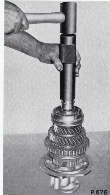
Fig. E.14. Fitting the spring ring in the mainshaft groove using Churchill Tool R.G.76 in conjunction with the hollow drift portion of R.G.77
