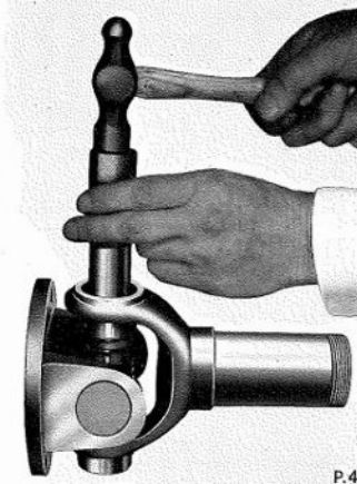
Fig. D.17. Removing the needle bearing cage
