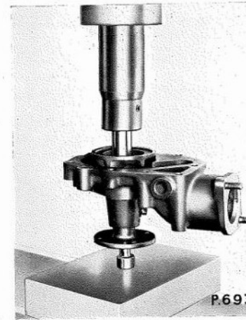
Fig. A.7. Pressing the impellor on to the bearing shaft
