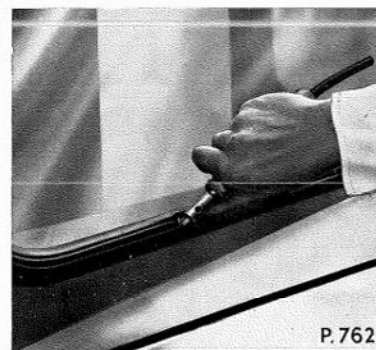
Fig. O.2. Refitting the rubber filler strip using a glazing tool
