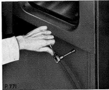
Fig. O.12. Releasing the front wing setscrews after removing the inner kicking trim panel
