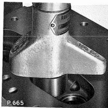
Fig. B.8. Correct location of the Churchill Adaptor R.G.10A-6 on the cylinder head valve seating, during valve guide removal
