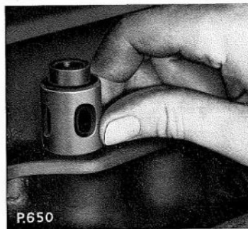
Fig. B.20. Withdrawing the tappets through the tappet chest aperture
