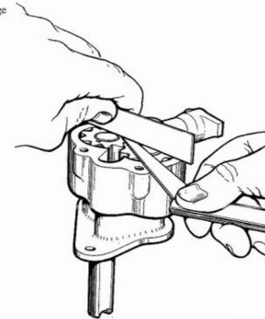
Fig. B.68. Checking oil pump gear end clearance, using a feeler gauge and straight edge
