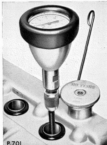
Fig. B.75. Checking the engine compression pressure, using the Churchill Tool 430, in conjunction with adaptor set 430-1
