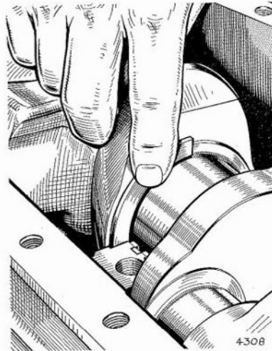
Fig. B.114. Installing the crankshaft thrust washers into the crankcase recesses at the rear intermediate main bearing position
