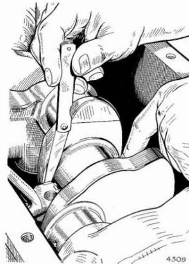
Fig. B.115. Checking the crankshaft end float using a feeler gauge
