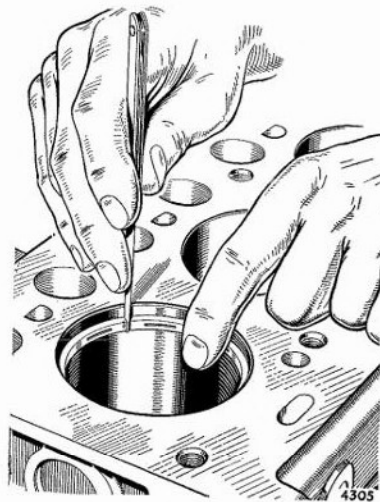
Fig. B.106. Checking the piston ring gap in the cylinder bore, using a feeler gauge
